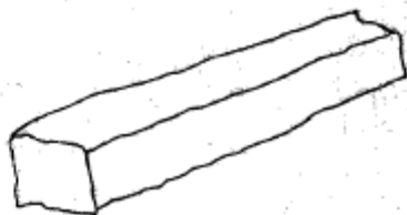
Exhibit 7.9 : Header or Bond Stone (Through Stone)
