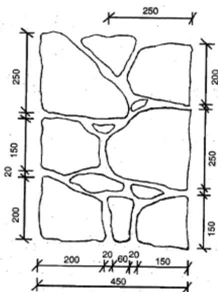
Exhibit 15.6 Alternative Correct, Method of Execution of Random Rubble Masonry using stones, of size as prescribed in Annexure 7.1
