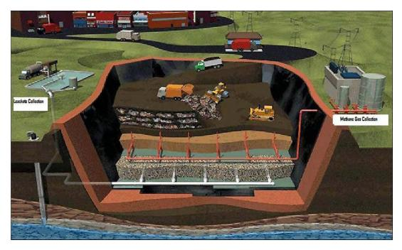
FIGURE 6.5: SCHEMATIC DIAGRAM OF LEACHATE CONTROL MECHANISM AT SANITARY LANDFILL
